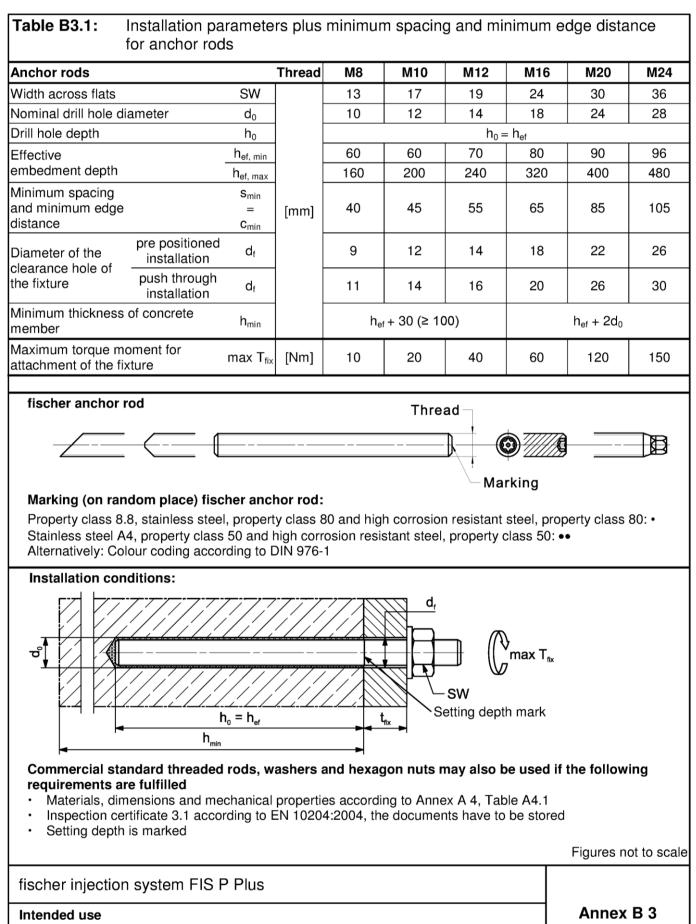
Installation parameters anchor rods
